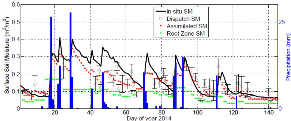
*Fig.5 - Assimilation of DISPATCH soil moisture data into a dynamic model for mapping irrigated areas and retrieving irrigation dates (Y. Malbêteau PhD thesis).*
